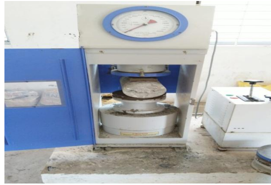
Figure 4. Compressive test on concrete
