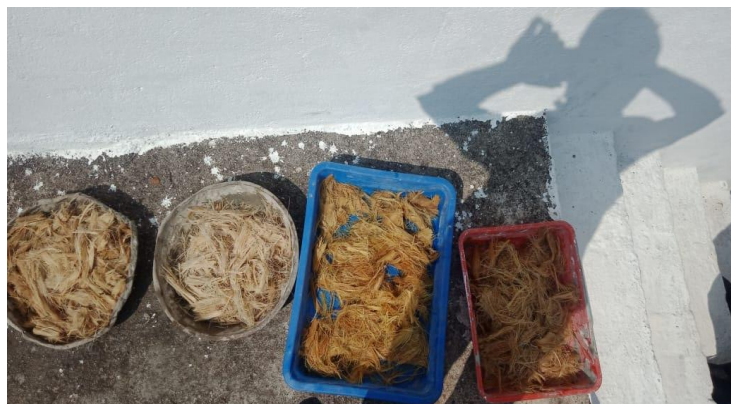
Figure 2. Banana Fiber treated in 1%, 2%, 3% and 6% of NaOH solution
