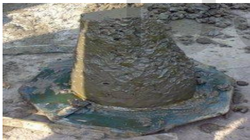
Figure 3. Slump Cone Test
